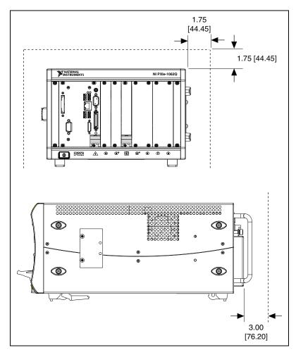
Figure 2-1. NI PXIe-1062Q Cooling Clearances
