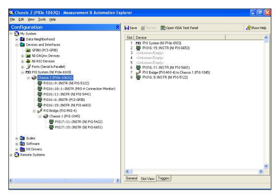
Figure 2-6. Multichassis Configuration in MAX
