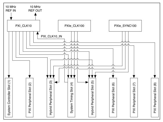
Figure 1-5. Distribution of PXI\_CLK10, PXIe\_CLK100, and PXIe\_SYNC100
