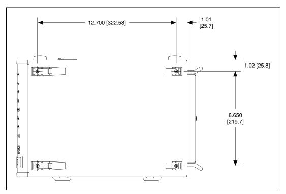
Figure A-2. NI PXIe-1062Q Chassis Dimensions (Bottom)
