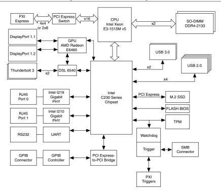
The PXIe-8861 consists of the following logic blocks on one circuit card assembly (CCA):
