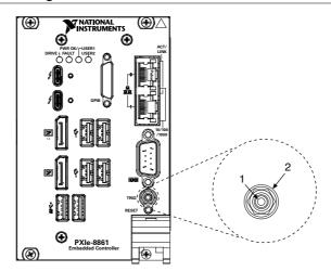
Figure 8. TRIG Connector Location and Pinout
